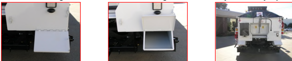
Left & Right Rear Shovel Outlets Fitted Only When Rear Spreaders are not Required
